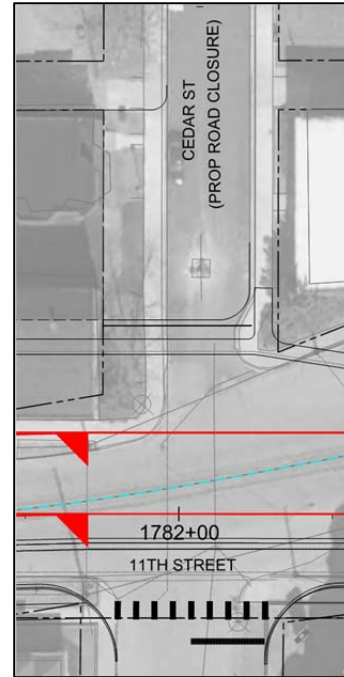
Figure 4-15. Proposed Improvements at the Intersection of 11 th and Cedar Streets
