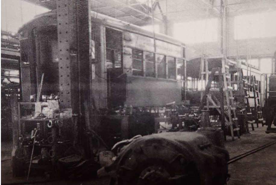
Figure 20. Improvements to SSL cars were undertaken locally in Michigan City shops. □ (Top) A car is cut in half for lengthening, (bottom) new "picture" windows are installed, c. 1940 (Middleton 1970: 154).
